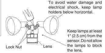
Adjust the lamp holders by loosening the lock nuts but do not rotate the lamp holders more than 180° from the factory setting. When screwing in the floodlamps, do not overtighten.
